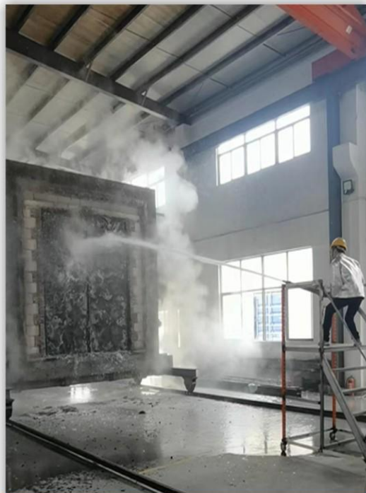
UL 10b&10c Fireproof and Hose Stream Test
